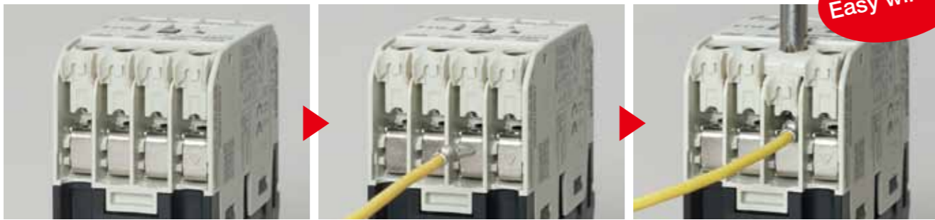
① Screw holder lifts up the screw.
